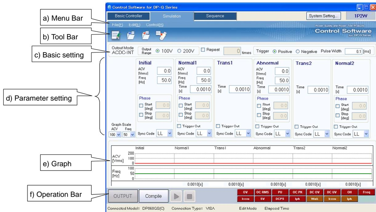
Figure 5-1 Simulation Window
