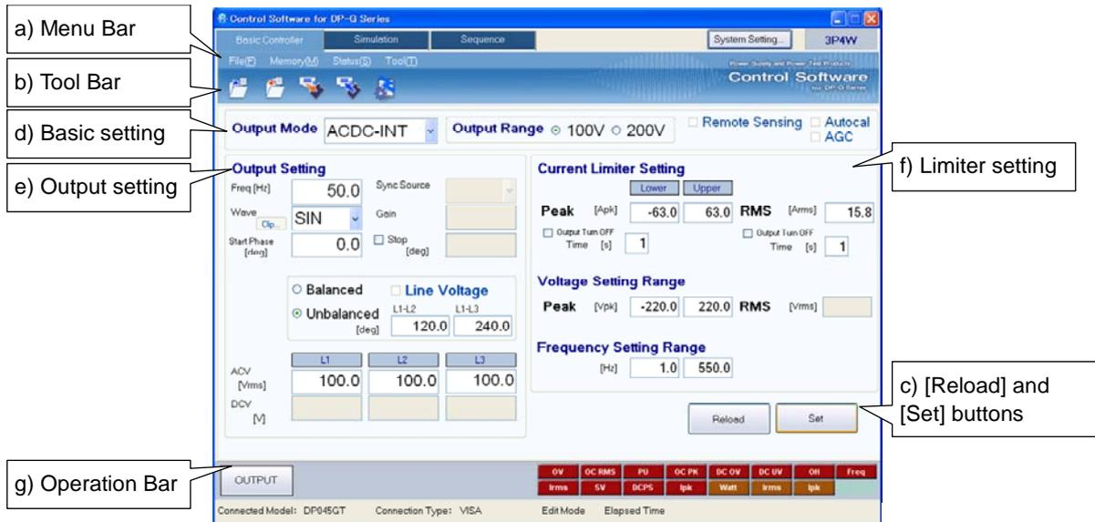
Figure 4-1 Basic Controller Window
