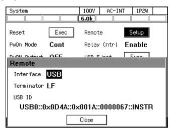
5. Use a commercially available USB cable (Type A to B) to connect this product to the computer. USB connector is available on the rear of this product.
