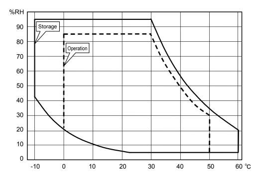
Figure 10-1 Range of Ambient Temperature/Humidity
