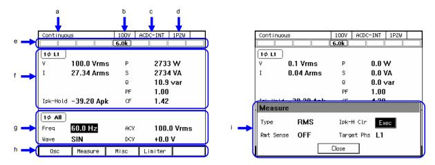
Figure 5-1 Component Name (Display Areas on the Screen)
