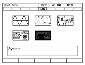
2. Put the cursor on [Setup] next to the [Remote] item, then press the ENTER key. The remote setting window opens.
