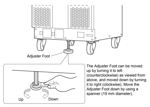
Figure 2-1 How to Use the Adjuster Foot
