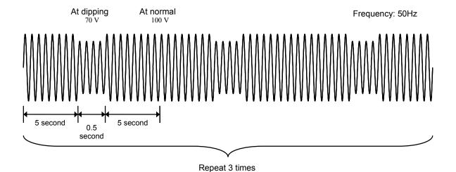
Figure 4-12 Voltage Dip Simulation Example
