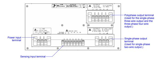
Figure 2-2 Terminal Panel Arrangement of Multi-phase Model (Rear)
