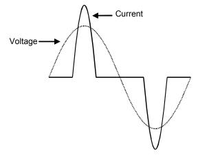
Figure 4-20 Current Waveform Containing Many Harmonic Components
