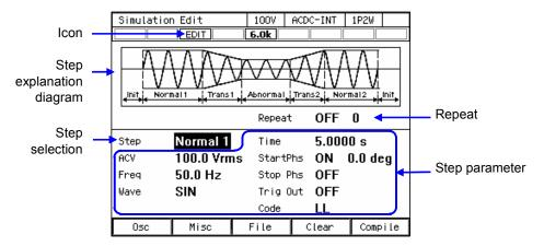
Figure 4-16 Simulation Edit View
