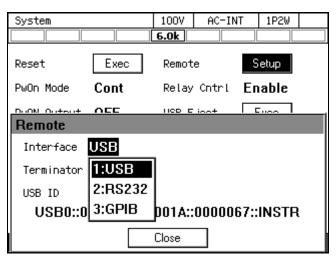
4. The window shows [Terminator] and [USB ID]. For the USB ID, see the explanation in the next section. Select [OK] to close the window.
