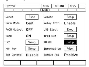
3. Enable/Disable the energization. The power unit on which the energization is enabled/disabled is represented by  $\square/\square$  respectively. Move the cursor to  $\square/\square$  and press the ENTER key to switch between  $\square$  and  $\square$ .
