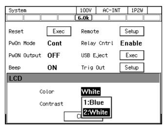
100V AC-INT 1P2W 6.0k Exec Setup Remote Reset Pw0n Mode Cont Relay Cotrl Enable PwON Output OFF USB Eject Exec ON Веер Trig Out Setup LCD Color Contrast Close
