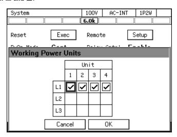
4. Select [OK]. The energization is enabled or disabled and the window is closed.
