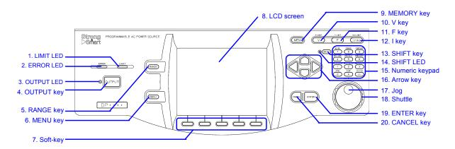
**Figure 3-3 Component Name (Control Panel)**
