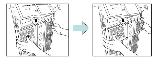
5. Remove the air filters from the back of each front grill. Be careful with the small claws on the front grill that hold the air filters.
