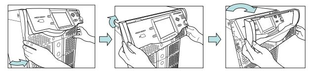
4. Each of the other front grills is fixed at the bottom left and right to the chassis. Hold it at the left and right sides, and pull it out toward you to remove it.
