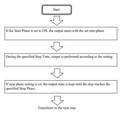
Figure 4-14 Process Flow through Simulation Steps
