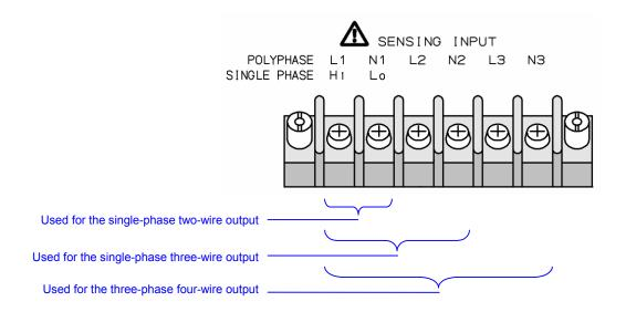
Figure 4-24 Sensing Input Terminals in Multi-phase Model
