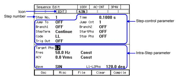
Figure 4-1 Step-control Parameters and intra-Step Parameters
