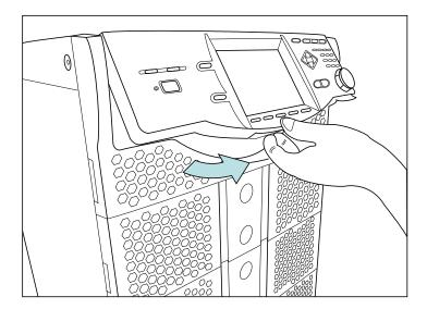
3. Dismount the front grills in turn from the top. The topmost front grill is fixed at the bottom left and right to the chassis, and hung at the top on the hook of the chassis. Hold the front grill at the bottom left and right sides, and pull it out toward you to release it. Move the front grill upward and toward you. Unhook and remove it as letting the control panel through it.
