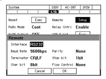
5. Use a D-sub 9-pin cross cable to connect this product to the computer. The connector is on the rear of this product.
