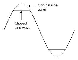
Figure 4-22 Clipped Sine Wave
