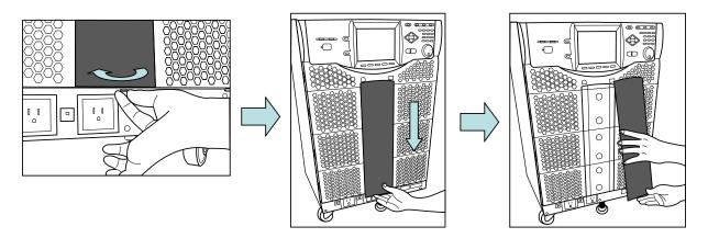
2. Flip up the control panel to its maximum angle.
