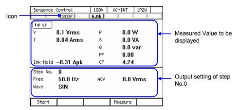
Figure 4-10 Sequence Control View (Output On State/Sequence Stopped)
