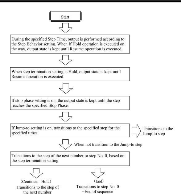
Figure 4-5 Process Flow in Sequence Step
