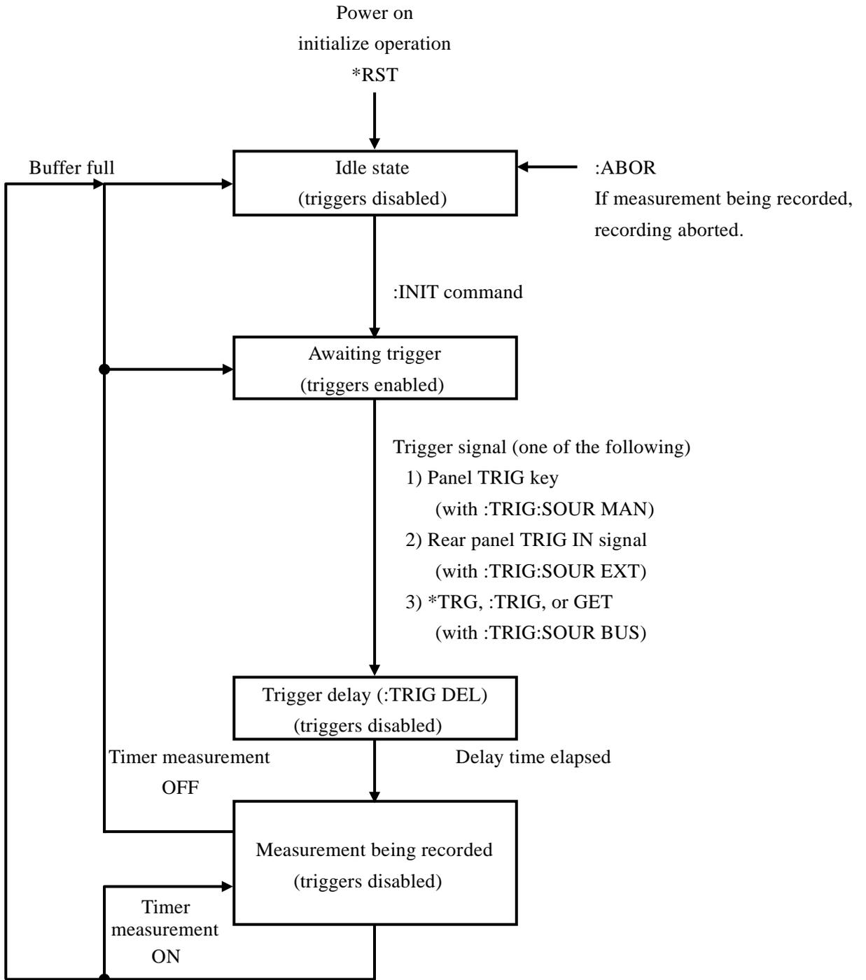
Fig. 7-1 Trigger system
