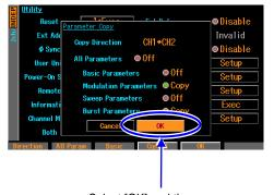
4. When the above setting is completed, select [OK] at the bottom of the window, and then press the ENTER key. The copy operation is performed. When you do not want to copy, select [Cancel] at the bottom of the window and press the ENTER key, or press the CANCEL key.
