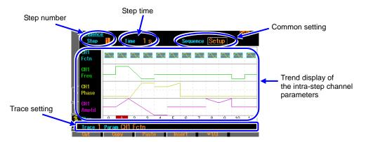
[PRM] and [SCL] displayed in the trace settings indicate the display item and the height of the trace frame, respectively. [OFS] indicates the bottom value of the trace frame for frequency, amplitude, and duty, and the center value of the trace frame for offset and phase.
