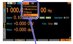
Press the MODE key to open the oscillation mode selection list. Select the burst oscillation mode [Burst]. (FP.4-27) This switches to burst oscillation mode.
