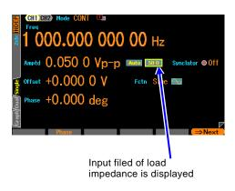
2. Select the desired load impedance condition, and then press the corresponding soft-key. When [Vari] is selected, the load impedance can be set. In this case, the input field of load impedance value is displayed to the right of the load impedance field.
