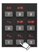
2. Pressing the key directly below the lighting waveform will select that waveform and reflect it in the output. For example, in the image shown to the left, pressing the [2] key will select the Square wave. Another method is to choose the selection list with the arrow keys or modify knob and then press ENTER to apply the settings.
