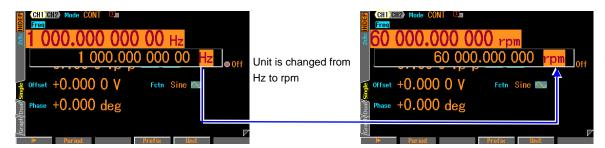
This can display and set a value in units of rpm.
