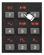
When you set the waveform as arbitrary wave, the arbitrary waveform stored in the main unit is selected. P.4-53
