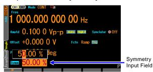
When the [Symm] field is selected and the ENTER key is pressed, the input field for pulse width time opens. [Symm] is displayed on the first page.
