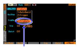
Select burst oscillation mode [BrstMode] on the second page of the setting screen, and press the ENTER key to display the burst mode selection list. Selecting triggered gate oscillation [TrigGate] will set the triggered gate oscillation mode.
