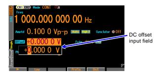
Press the shortcut-key OFFSET to open the DC offset input field. Or select the [Offset] field and then press the ENTER key to open the DC offset input field. [Offset] is displayed at the top left on the first page.
