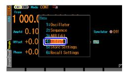
When the MENU key is pressed, the top menu opens. Then, press the soft-key corresponding to [UTILITY]. This opens the Utility.
