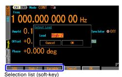
When the load impedance field at the right of the range field is selected and the ENTER key is pressed, the selection list is displayed.
