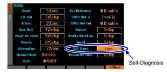
Self-diagnosis checks the internal status. Since the check stops the oscillation and turns off the output, it is recommended to initialize the setting by [Reset] in advance.
