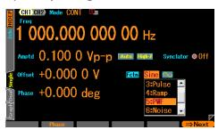
Press the FCTN key to display the waveforms above the numeric keypad and select the key ([5] key) corresponding to the PWF. The waveform which is currently set as the PWF is output. Similar to other waveforms, the waveform's polarity and amplitude range may also be changed.
