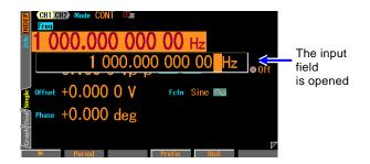
2. Press the ENTER key to open an entry field to change the current value. In this state, you can enter a value using the numeric keypad.
