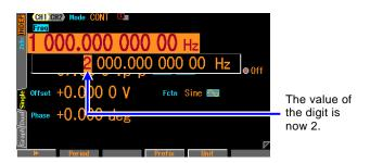
Increment or decrement the value of the digit using the up/down arrow keys or the modify knob.
