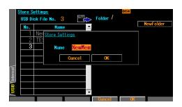
2. When saving to USB, first connect the USB flash memory to the unit, then select the USB tab on the far left of the screen and press the ENTER key. In the Store Settings screen, select the [USB Disk File No.] field on the top left of the screen, and then press the ENTER key to open the input field of the setting memory number to be saved. Use the up/down arrow keys or the modify knob to increment or decrement the setting memory
