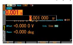
When the input field of Period appears, set in the same way as the one for Frequency. When a number is entered by using the numeric keypad, the unit key for period setting is displayed on the soft-key. When changed to the period display, the displayed is changed as follows.
