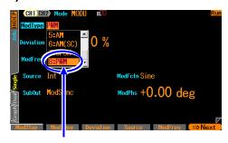
Set the modulation type [ModType] to PWM [PWM] on the second page of the setting screen when the oscillation mode [Mode] is set to modulation [MODU] and on the third page of the setting screen when the mode is burst [BURST] or sweep [SWEEP].
