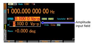
Press the shortcut-key AMPTD to open the amplitude input field. Or select the [Amplitude] field and then press the ENTER key.
