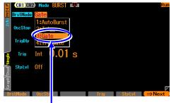
press the ENTER key to display the burst mode selection list. Selecting gate oscillation [Gate] sets the gate oscillation mode.
