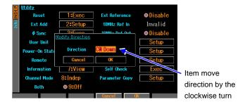
Select whether the item selection moves up or down when you turn the modify knob clockwise (CW) while the channel mode selection list is displayed.
