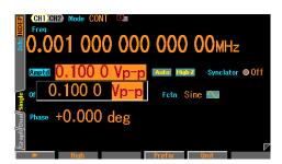
1. Select amplitude and then press the ENTER key to open the input field.
