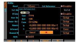
Type: Freq Unit: rpm Form: (h+n)\*m
