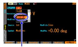
Set the modulation type [ModType] to DC offset modulation [OFSM] on the second page of the setting screen when the oscillation mode [Mode] is set to modulation [MODU] and on the third page of the setting screen when the mode is burst [BURST] or sweep [SWEEP].
