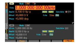
The channel to be set can be switched by using the CH1/CH2 key.
