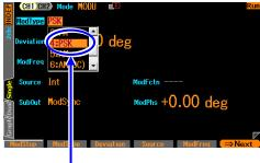
Set the modulation type [ModType] to PSK [PSK] on the second page of the setting screen when the oscillation mode [Mode] is set to modulation [MODU] and on the third page of the setting screen when the mode is sweep [SWEEP].
