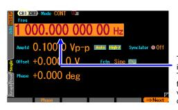
The frequency is selected. The current frequency value is displayed.  Select the desired item with the arrow keys or the modify knob.
