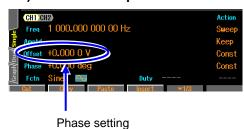
If the waveform of the previous step is DC or noise, oscillation in the next step starts from reference phase  $0^{\circ}$ . Phase  $0^{\circ}$  here is the phase value based on the reference phase as in the case of the phase at step end (stop phase). The start phase that appears in the actual output is the phase setting value of that step. If the phase is set to  $0^{\circ}$ , oscillation starts from  $0^{\circ}$ .
